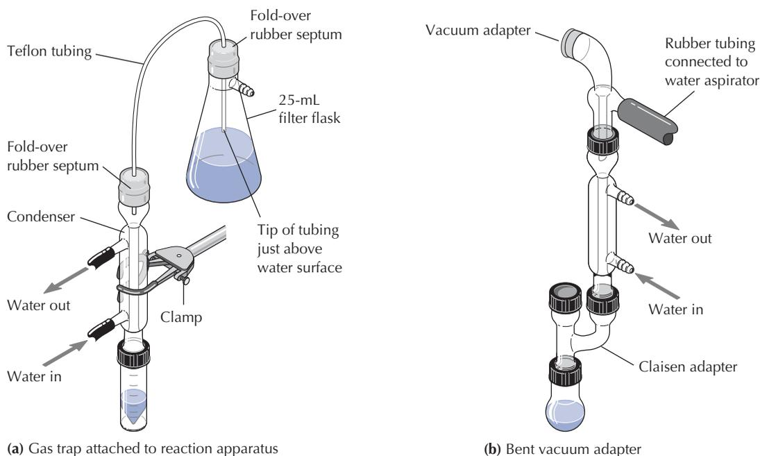
**FIGURE 7.8** Standard taper microscale apparatus used to trap water-soluble noxious vapors.
