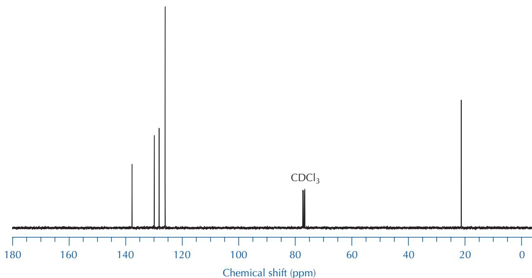
**FIGURE 22.3** Broadband-decoupled 90-MHz  $^{13}\text{C}$  NMR spectrum of an aromatic compound with molecular formula  $\text{C}_8\text{H}_{10}$  in  $\text{CDCl}_3$ .
