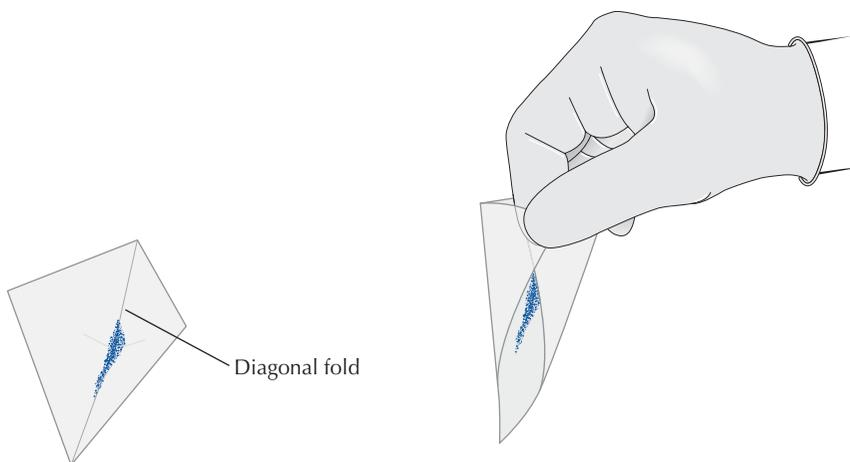
(a) Diagonally folded weighing paper with a solid sample (b) Overlap opposite diagonal corners and hold firmly between thumb and index finger.
