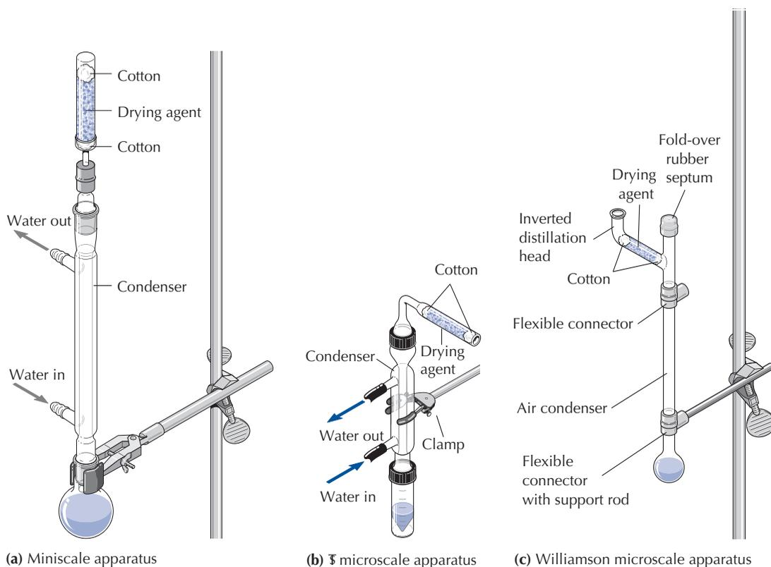
FIGURE 7.2 Refluxing under anhydrous conditions.
