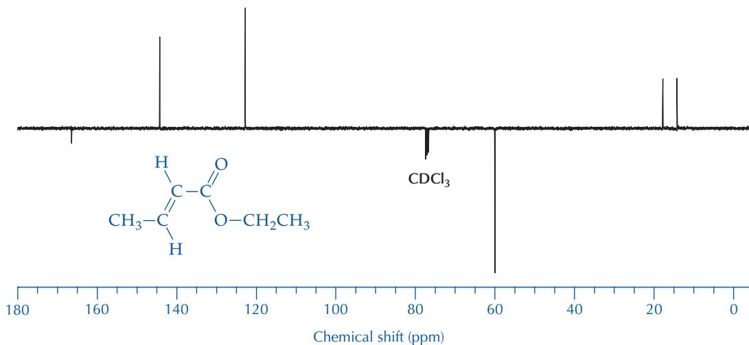
**FIGURE 22.10** 90-MHz  $^{13}\text{C}$  NMR spectrum of ethyl *trans*-2-butenoate in  $\text{CDCl}_3$  using an APT pulse sequence.
