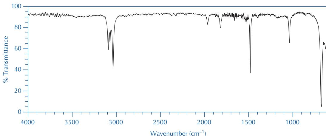
FIGURE 20.31 IR spectrum for question 4 (thin film).
