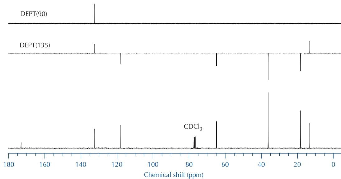
**FIGURE 25.17** 90-MHz <sup>13</sup>C NMR, DEPT(90), and DEPT(135) spectra of unknown compound for problem 8.
