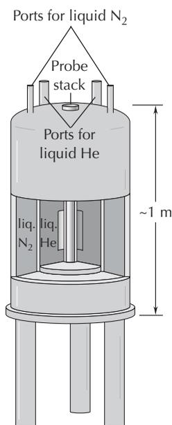
**FIGURE 21.6** Typical superconducting electromagnet for a 200- to 400-MHz NMR spectrometer, showing the vacuum-jacketed Dewar vessels for the liquid nitrogen and liquid helium coolants.
