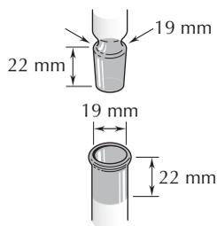
FIGURE 4.3 Dimensions of  $\text{19/22}$  ground glass joints.
