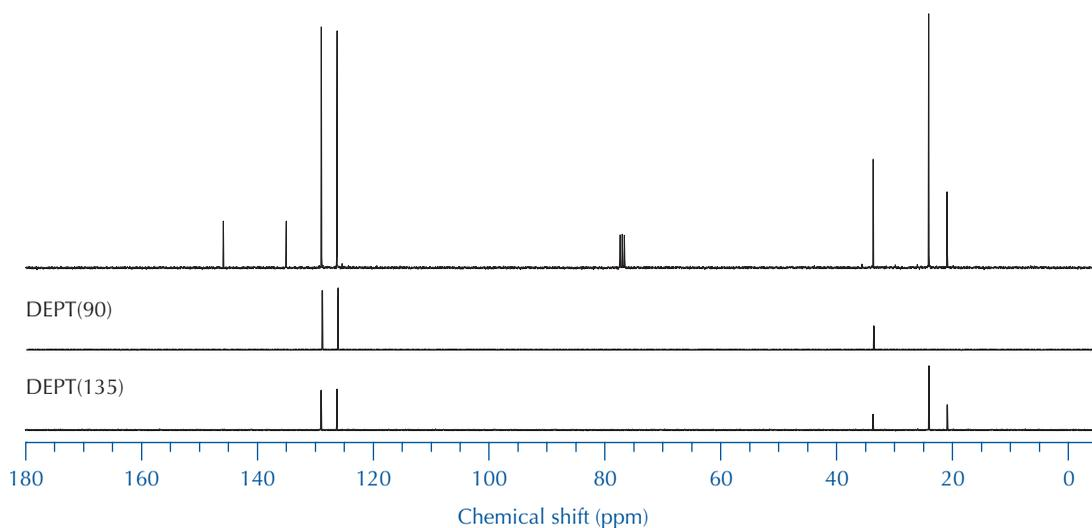
**FIGURE 22.17** 90-MHz  $^{13}\text{C}$  NMR, DEPT(90), and DEPT(135) spectra of a compound with molecular formula  $\text{C}_{10}\text{H}_{14}$ .
