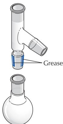
**FIGURE 4.5** Apply two *thin* strips of grease almost the entire length of the inner joint about 180° apart.
