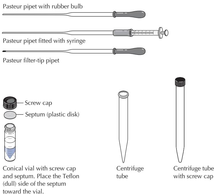
**FIGURE 11.6** Equipment for microscale extractions.
