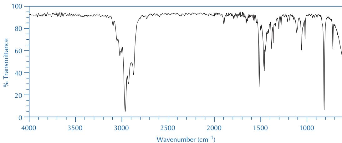
FIGURE 20.38 IR spectrum for question 5 (thin film).
