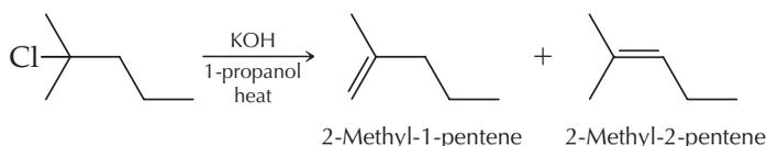
The expected products of the reaction are 2-methyl-1-pentene and 2-methyl-2-pentene, and it is quite possible that they will be contaminated with a small amount of 1-propanol, the solvent used in the reaction. The singlet at 2.2 ppm and the triplet at 3.6 ppm are produced by the hydroxyl proton of 1-propanol and the methylene group attached to the hydroxyl group. The other signals of 1-propanol, at 1.55 ppm and 0.92 ppm, are obscured by signals of the two alkenes.
