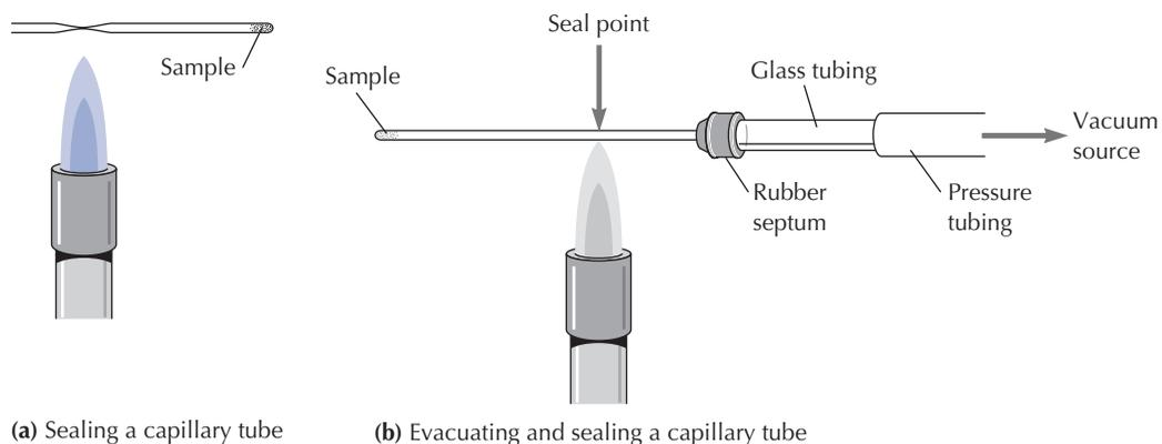
FIGURE 14.4 Methods for sealing a capillary tube with a Bunsen burner.
