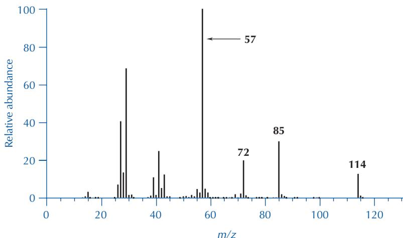
FIGURE 23.15 Mass spectrum of unknown for case study.
