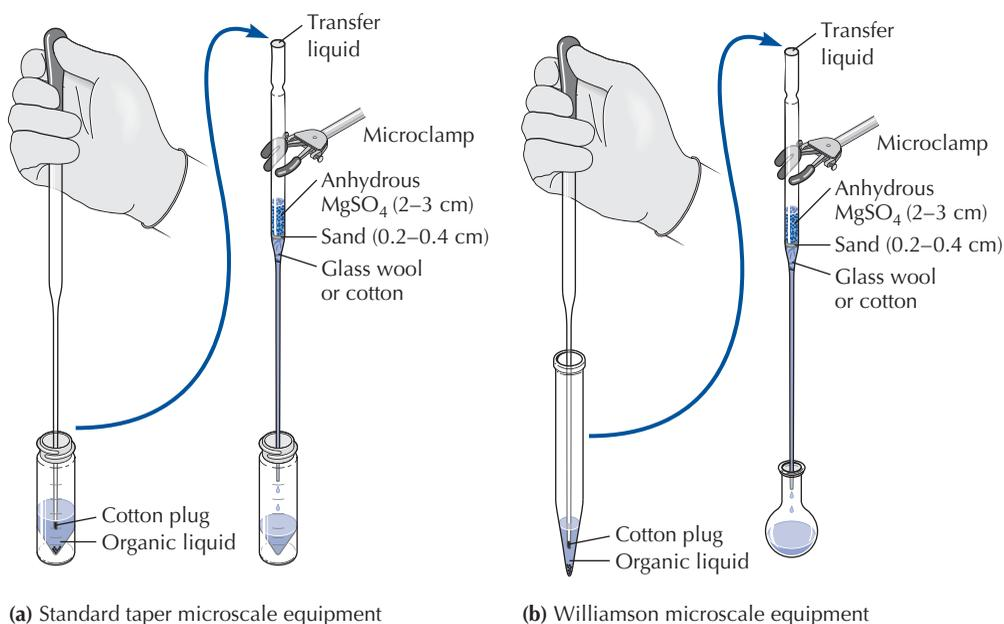
**FIGURE 12.4** Using microscale equipment and a Pasteur filter pipet containing anhydrous  $\text{MgSO}_4$  to dry an organic liquid or solution.
