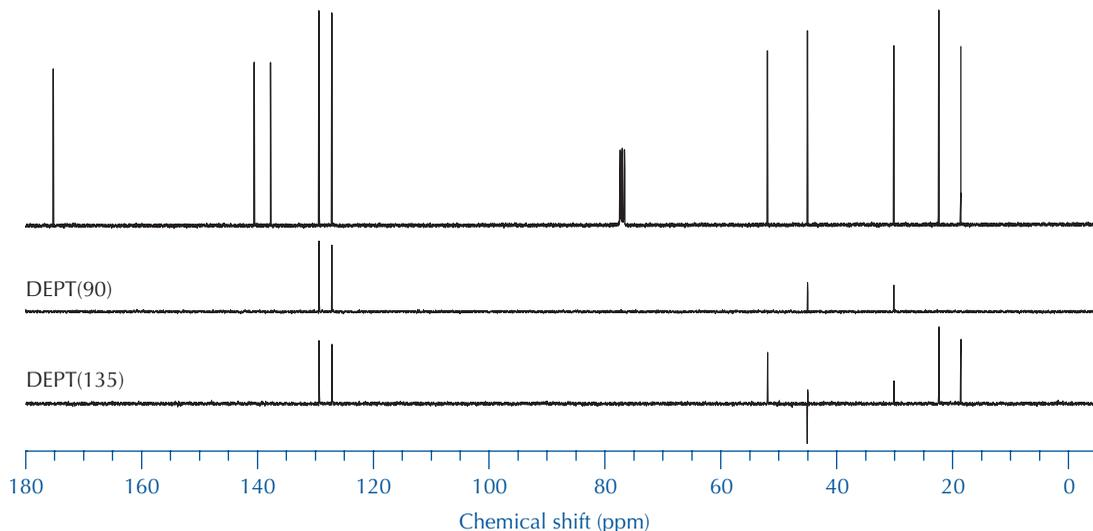
**FIGURE 22.19** 90-MHz  $^{13}\text{C}$  NMR, DEPT(90), and DEPT(135) spectra of the methyl ester of ibuprofen.
