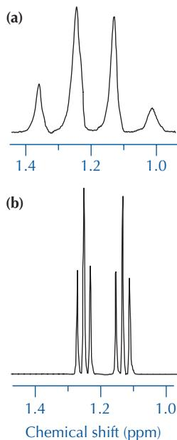
**FIGURE 21.31**  $^1\text{H}$  NMR spectra of the methyl group signals of ethyl propanoate at (a) 60 MHz and (b) 360 MHz.
