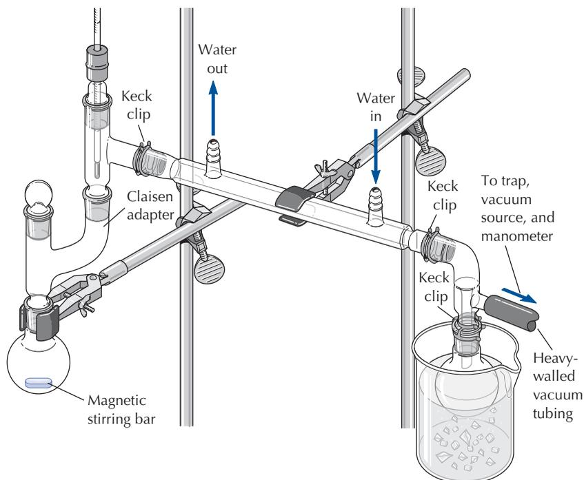
**FIGURE 13.26** Vacuum distillation apparatus.
