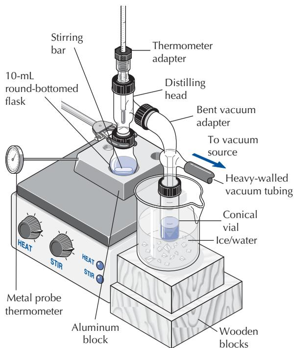
**FIGURE 13.28** Short-path standard taper microscale apparatus for vacuum distillation.
