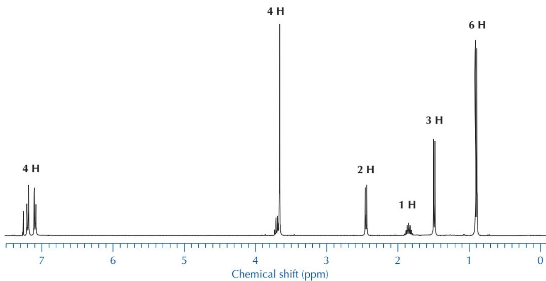
FIGURE 22.20 360-MHz  $^1\text{H}$  NMR spectrum of the methyl ester of ibuprofen.
