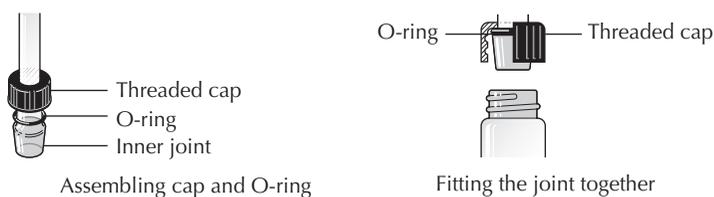
Figure 4.8. This type of microscale glassware fits together with flexible elastomeric connectors that are heat and solvent resistant.
