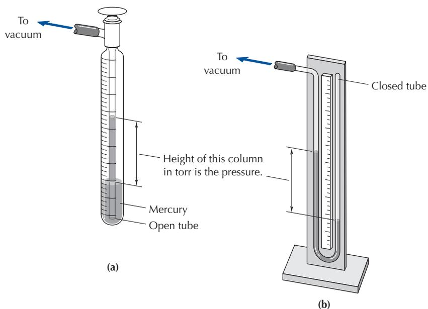
**FIGURE 13.23** Two types of closed-end manometers used in vacuum distillations.
