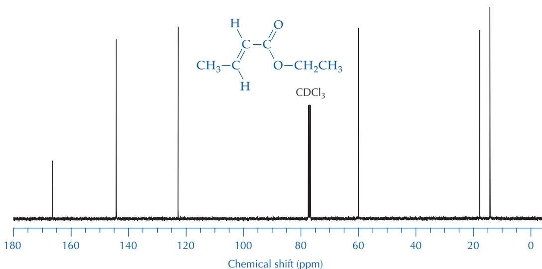
FIGURE 22.2 Broadband-decoupled 90-MHz  $^{13}\text{C}$  NMR spectrum of ethyl *trans*-2-butenoate in  $\text{CDCl}_3$ .
