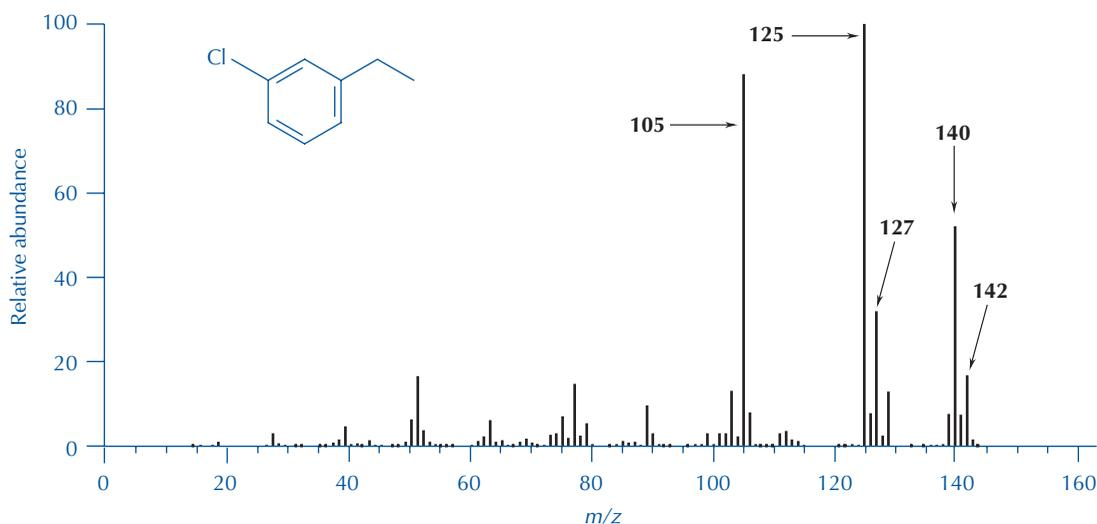
FIGURE 23.8 Mass spectrum of 3-chloroethylbenzene.
