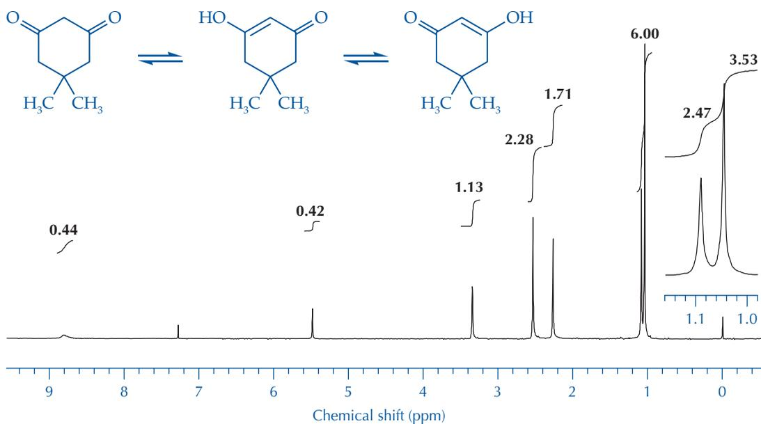
FIGURE 21.40 200-MHz  $^1\text{H}$  NMR spectrum of 5,5-dimethylcyclohexan-1,3-dione.
