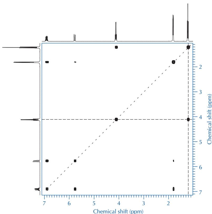
**FIGURE 22.13** 2D (H,H) COSY spectrum of ethyl *trans*-2-butenate in  $\text{CDCl}_3$ . The 1D 360-MHz  $^1\text{H}$  NMR spectra are shown at the top and left edges.
