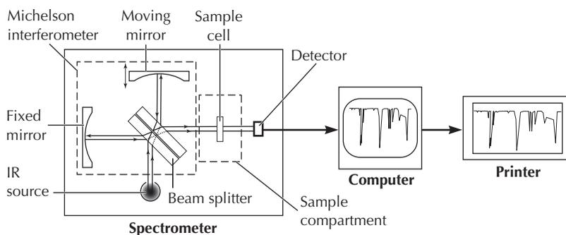
**FIGURE 20.6** Diagram of a single-beam FTIR spectrometer. The interior of the instrument is isolated from the ambient environment by purging with dry nitrogen or dry, carbon dioxide-free air.
