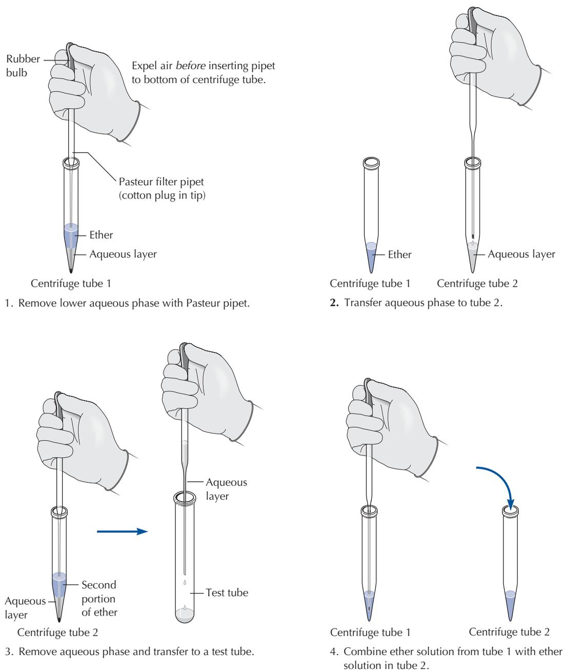
**FIGURE 11.8** Extracting an aqueous solution with an organic solvent less dense than water.
