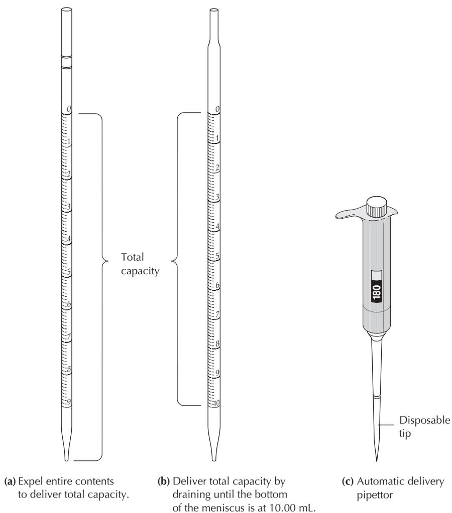
**FIGURE 5.7** (a and b) Types of graduated pipets. (c) Automatic delivery pipettor.
