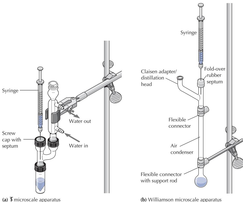
FIGURE 7.5 Using a syringe to add reagents to a microscale reaction.
