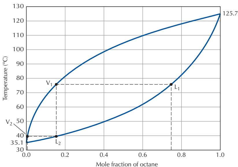
**FIGURE 13.6** Calculated temperature/composition diagram for pentane/octane solutions at 1.0 atm pressure.
