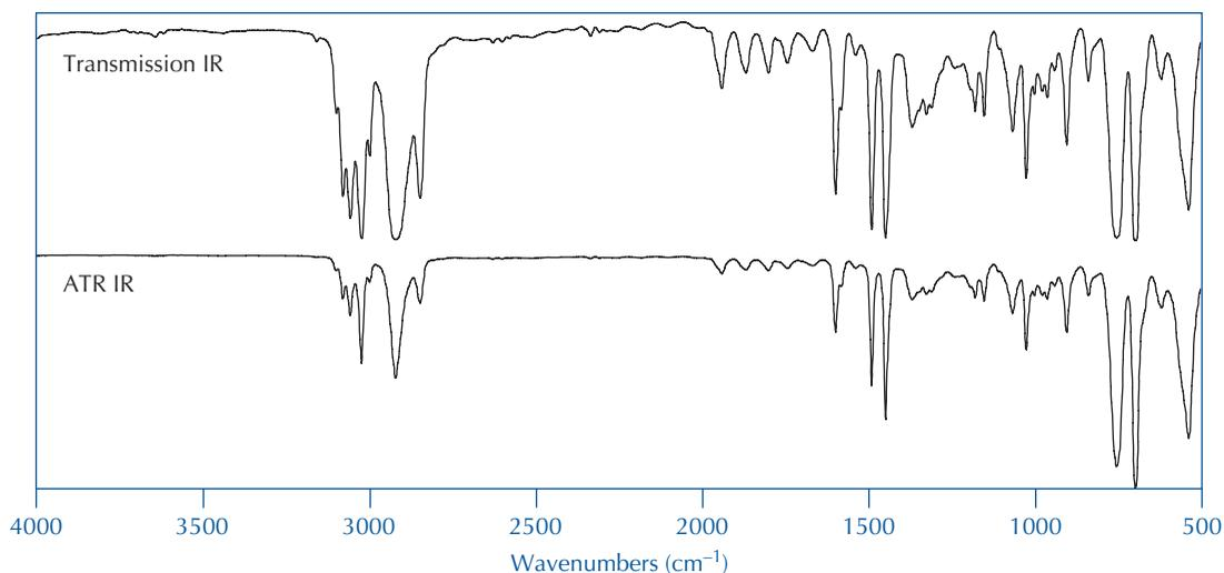
**FIGURE 20.13** Comparison of (top) a transmission spectrum of polystyrene with (bottom) an ATR spectrum of polystyrene.
