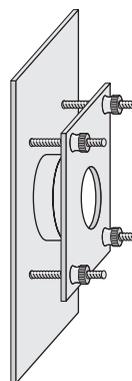
**FIGURE 20.9** IR sample disk holder for low-viscosity liquids. The holder slips into a bracket on the IR spectrometer.
