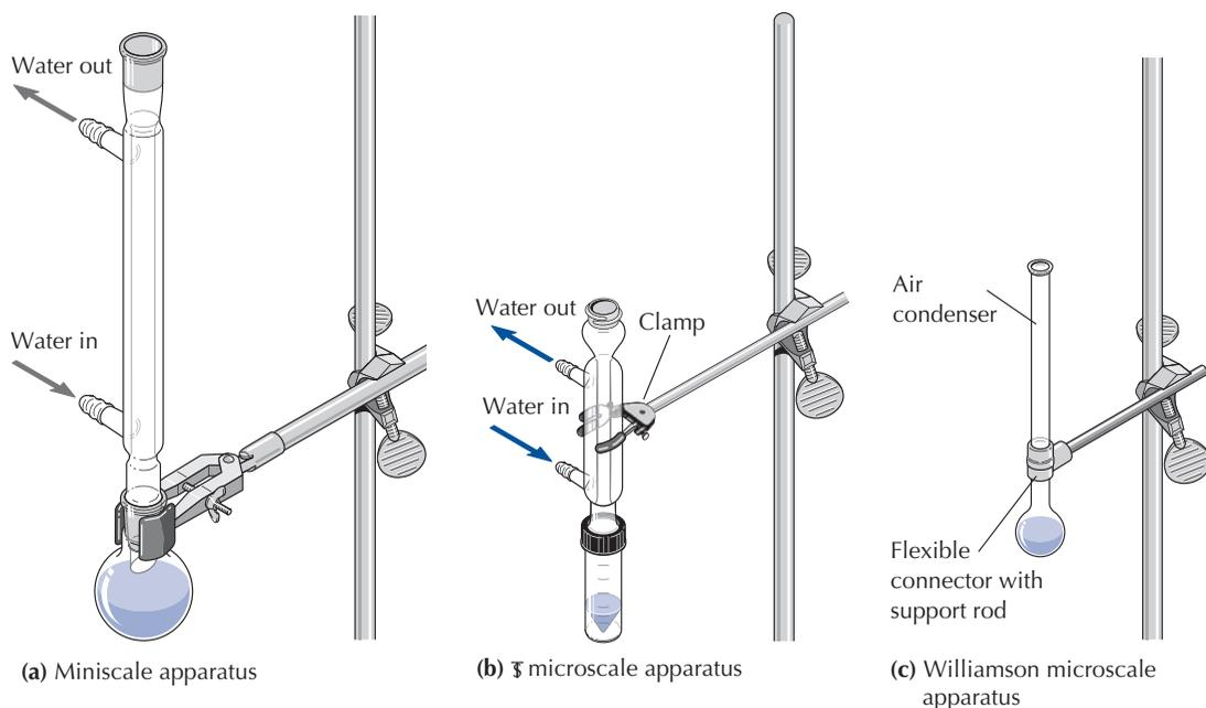
FIGURE 7.1 Apparatus for simple reflux.
