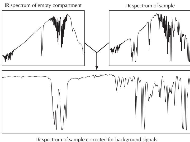
**FIGURE 20.7** The collection and processing of data required for the creation of an infrared spectrum with a single-beam FTIR spectrometer.
