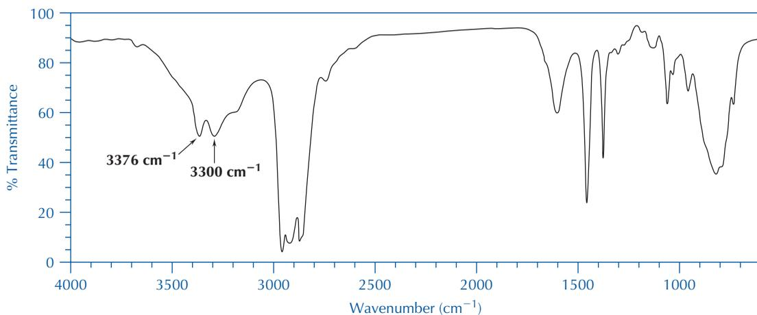
**FIGURE 25.11** Infrared spectrum (thin film) of unknown compound for problem 7.
