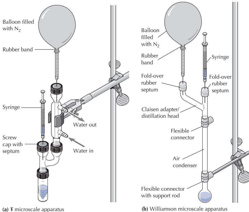
**FIGURE 16.10** Microscale reaction apparatus with balloon assembly for inert atmosphere conditions.
