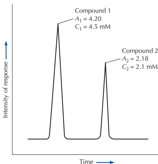
**FIGURE 19.13** Chromatogram of a standard mixture containing known concentrations of two compounds.
