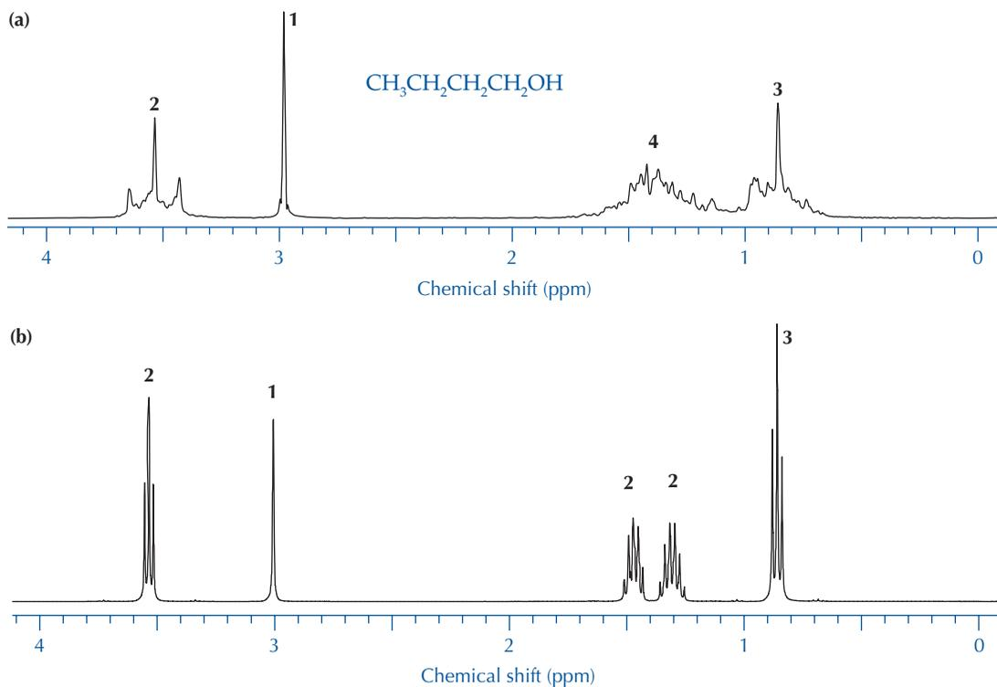
**FIGURE 21.30**  $^1\text{H}$  NMR spectra of 1-butanol at (a) 60 MHz and (b) 360 MHz.
