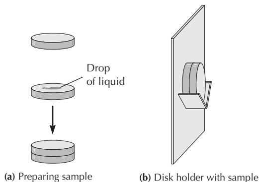
**FIGURE 20.8** Preparation of thin-film sample for IR spectroscopy.
