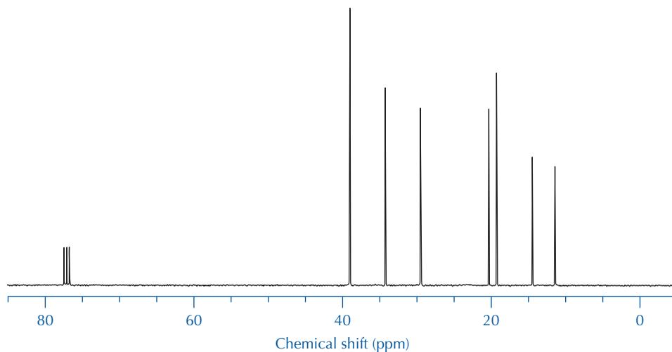
**FIGURE 22.8** Broadband-decoupled 90-MHz  $^{13}\text{C}$  NMR spectrum of 3-methylhexane in  $\text{CDCl}_3$ .
