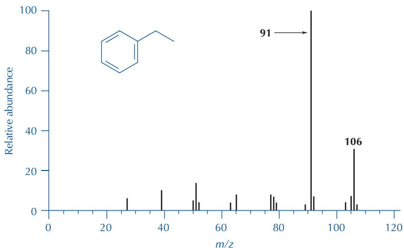
**FIGURE 23.11** Mass spectrum of ethylbenzene.
