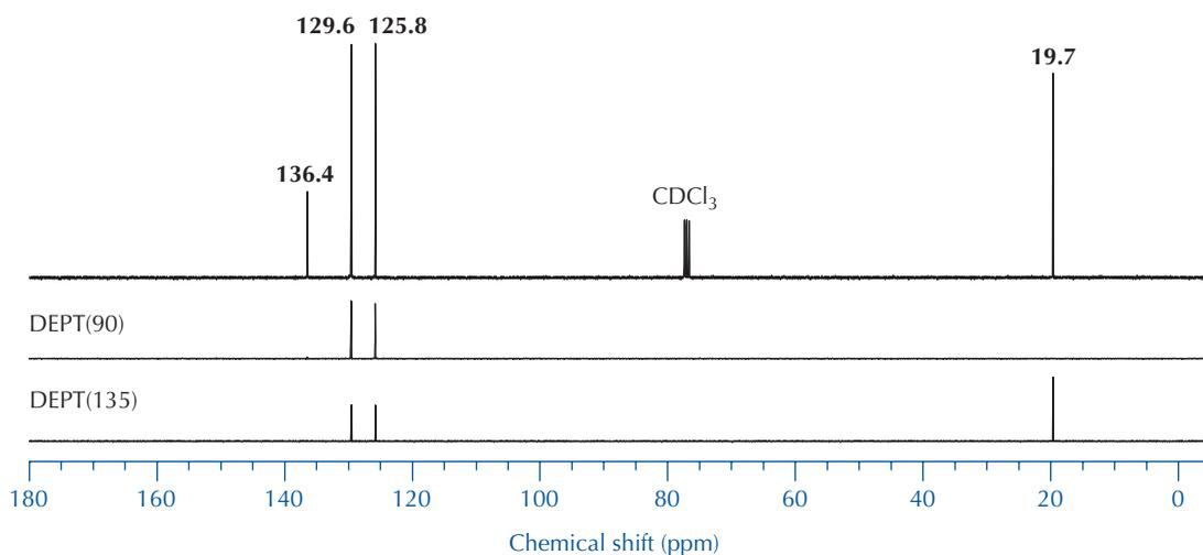
**FIGURE 22.16** 90-MHz  $^{13}\text{C}$  NMR, DEPT(90), and DEPT(135) spectra of a compound with molecular formula  $\text{C}_8\text{H}_{10}$ .
