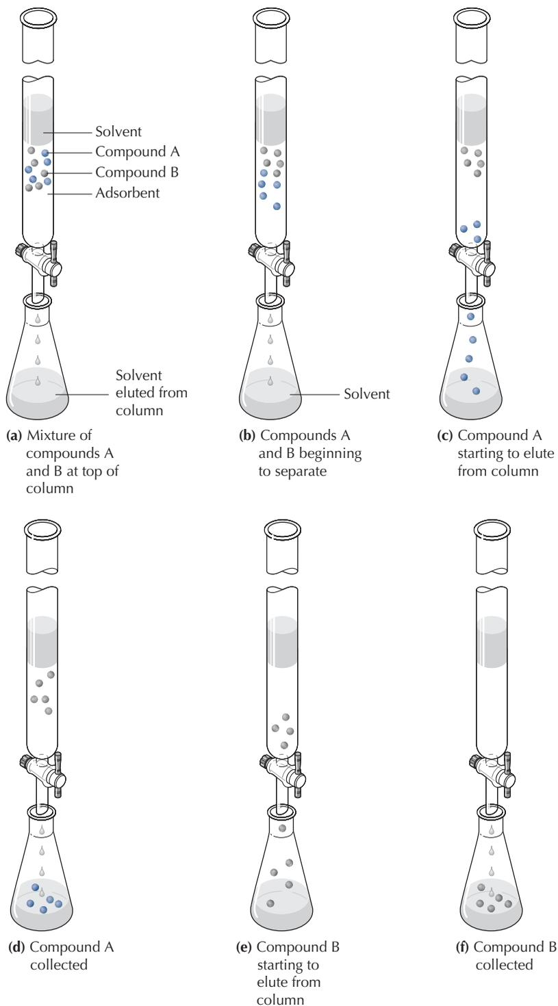
**FIGURE 18.1** Stages in liquid chromatographic separation of a mixture containing compound A and compound B. Compound A moves faster than does compound B, which is more strongly adsorbed on the stationary phase.
