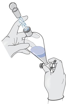
**FIGURE 11.4** Failure to vent the separatory funnel when extracting with  $\text{Na}_2\text{CO}_3$  or  $\text{NaHCO}_3$  solution can cause the stopper to pop out.
