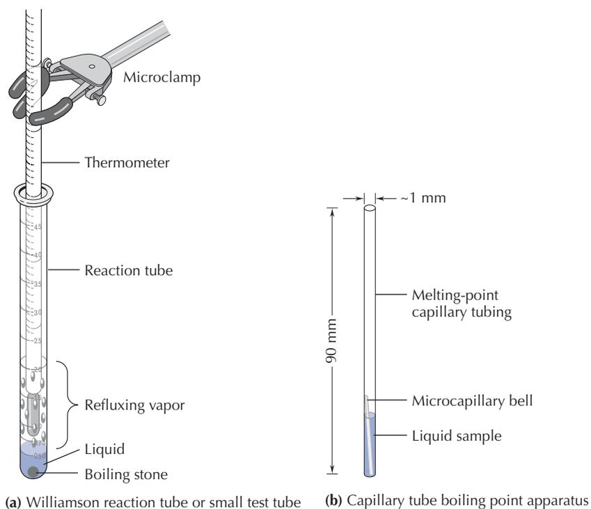
**FIGURE 13.2** Apparatus for microscale boiling-point determinations.
