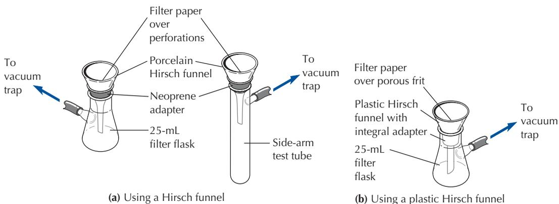
FIGURE 15.5 Vacuum filtration using a Hirsch funnel.
