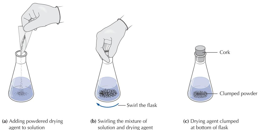
FIGURE 12.1 Adding drying agent to a solution.
