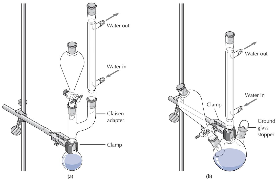
**FIGURE 7.4** Assemblies for adding reagents to a reaction heated under reflux in (a) a one-necked reaction flask and (b) a three-necked flask.
