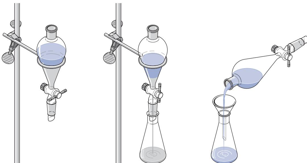
5. Use a ring stand to hold separatory funnel until layers separate.
