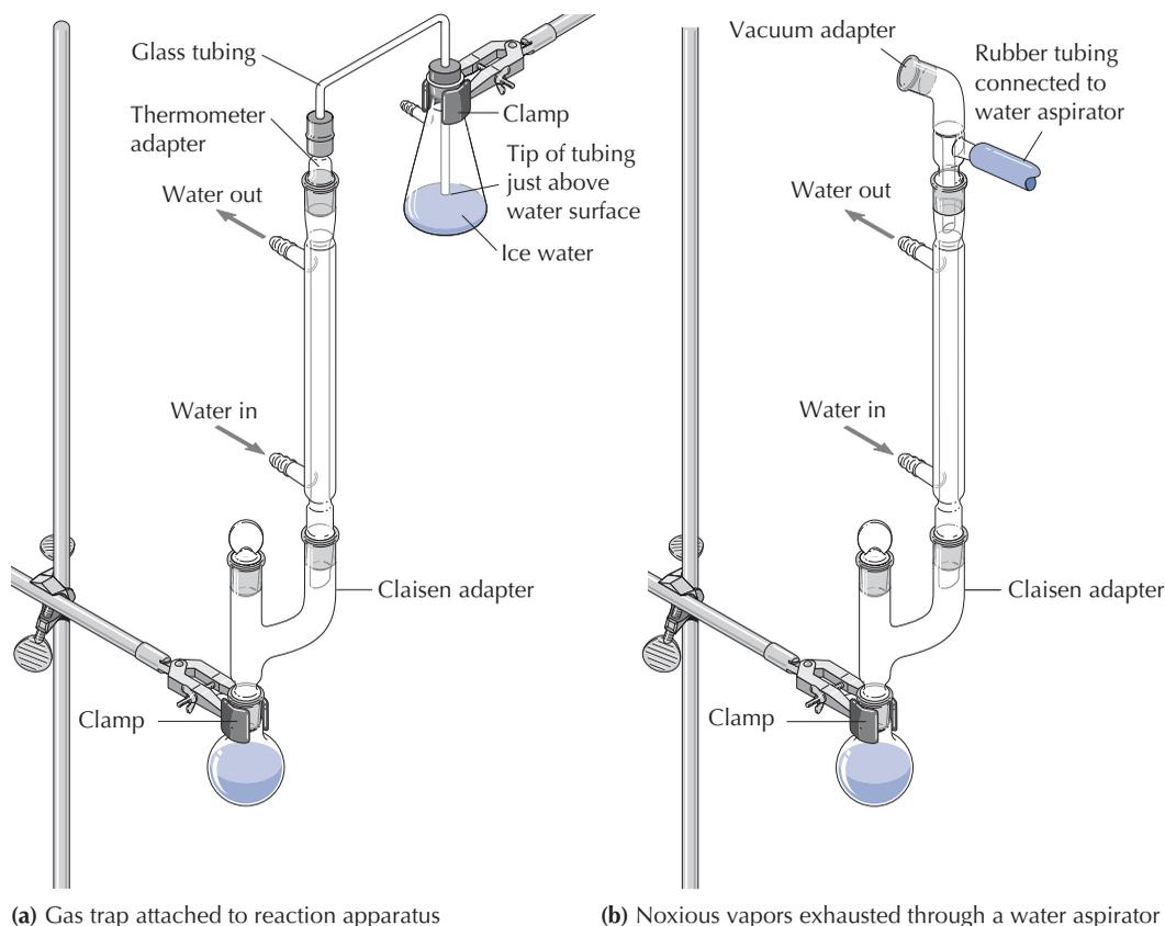
FIGURE 7.6 Miniscale apparatus used to trap water-soluble noxious vapors.
