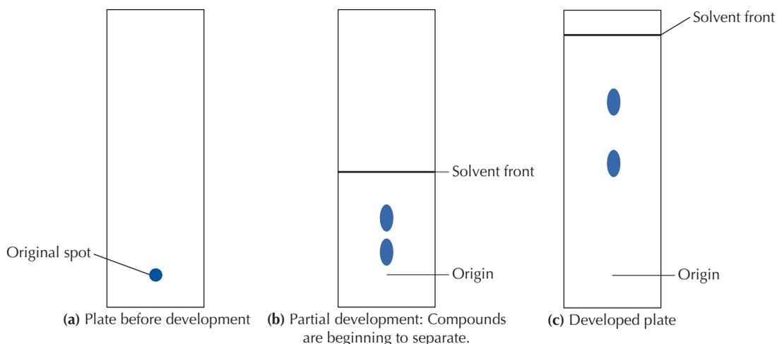
FIGURE 17.2 Steps in development of a TLC plate.
