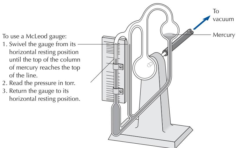
**FIGURE 13.24** McLeod gauge used in vacuum distillations, shown in the vertical measuring position.
