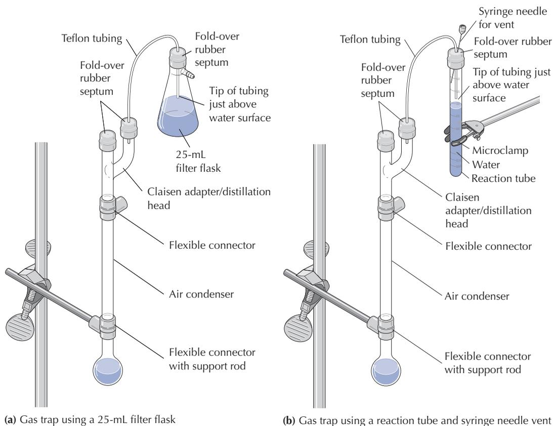
FIGURE 7.9 Williamson microscale apparatus used to trap water-soluble noxious vapors.
