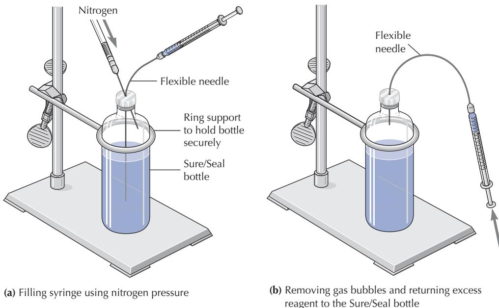
**FIGURE 16.11** Filling a syringe with an air-sensitive reagent. Reprinted with permission from Aldrich Chemical Co., Inc., Milwaukee, WI.
