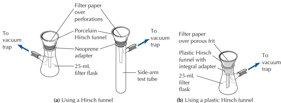
FIGURE 10.7 Microscale apparatus for vacuum filtration.
