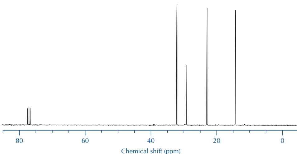
**FIGURE 22.7** Broadband-decoupled 90-MHz  $^{13}\text{C}$  NMR spectrum of heptane in  $\text{CDCl}_3$ .
