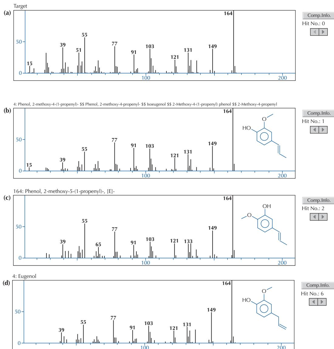
**FIGURE 23.18** Computer comparison of three hit list compounds for clove oil. (a) MS of the compound from the GC-MS run. (b) MS of hit 1. (c) MS of hit 2. (d) MS of hit 6.
