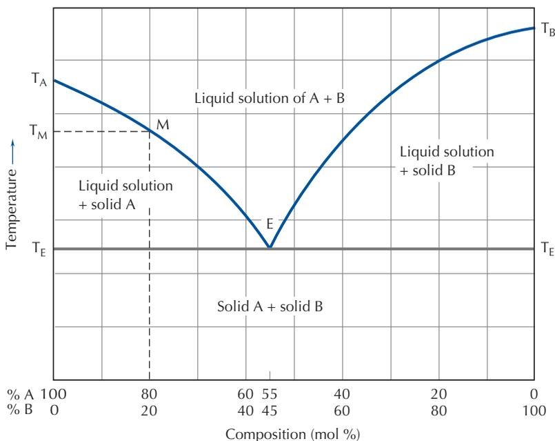
**FIGURE 14.1** Melting-point composition diagram for the binary mixture A + B.  $T_A$  is the melting point of pure solid A,  $T_B$  of pure solid B, and  $T_E$  of eutectic mixture E. The temperature range  $T_E - T_M$  is the melting range of a solid containing 80 mol % A and 20 mol % B.
