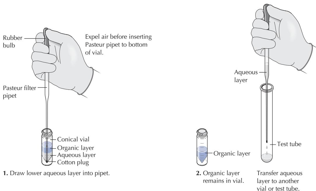
FIGURE 11.9 Washing an organic phase less dense than water.
