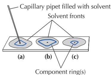
**FIGURE 17.9** Rapid method for determining an effective TLC solvent: (a) good development; (b) and (c) poor development.
