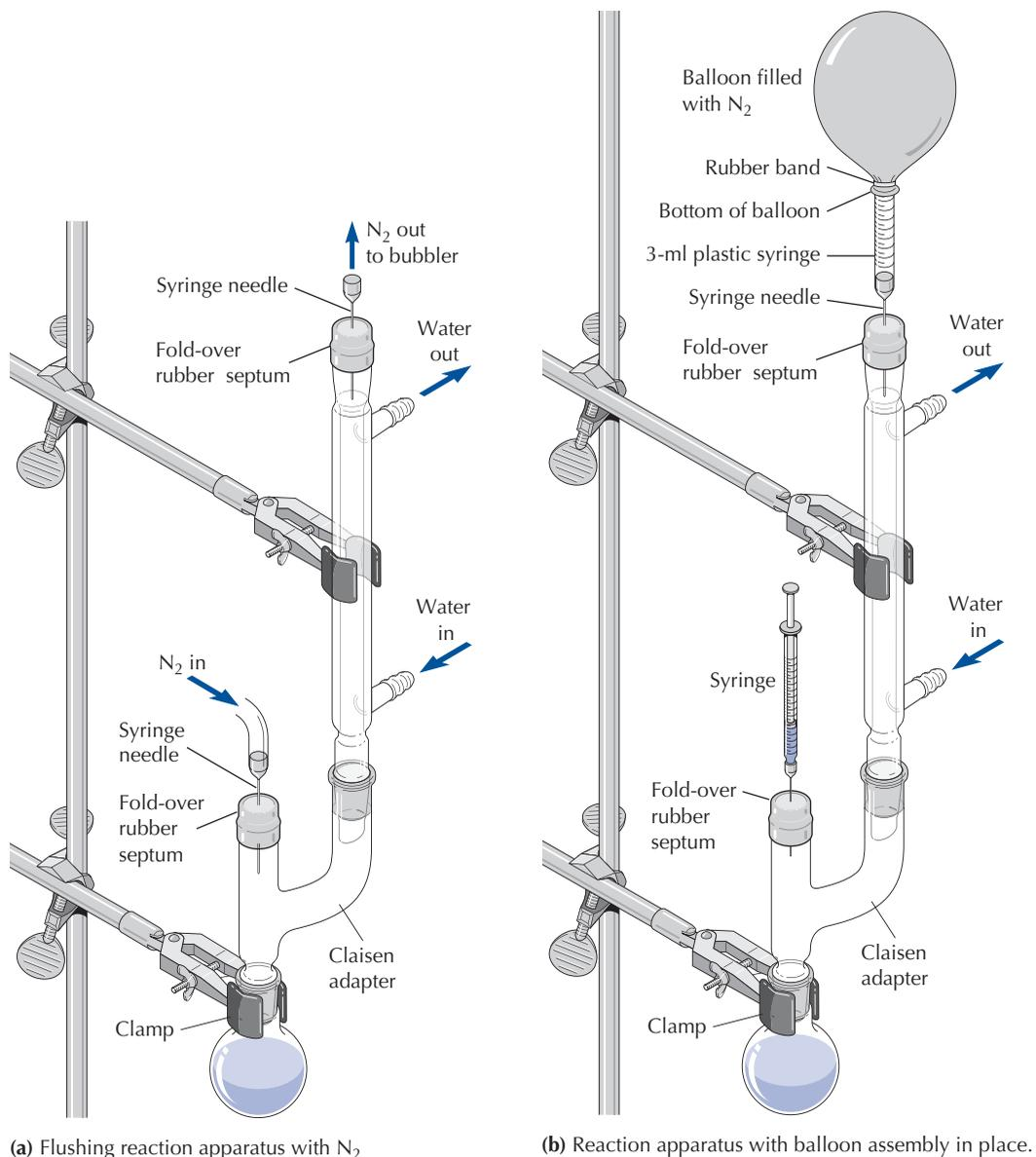
FIGURE 16.9 Miniscale reaction setups for inert atmosphere reaction conditions.
