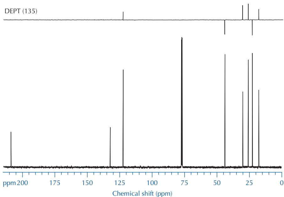
**FIGURE 22.12** The 90-MHz DEPT(135) and  $^{13}\text{C}$  NMR spectra of  $\text{C}_8\text{H}_{14}\text{O}$  in  $\text{CDCl}_3$ .
