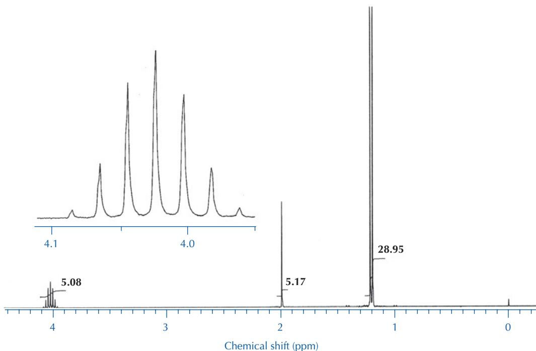
FIGURE 21.39 300-MHz  $^1\text{H}$  NMR spectrum of a compound of molecular formula  $\text{C}_3\text{H}_8\text{O}$ .
