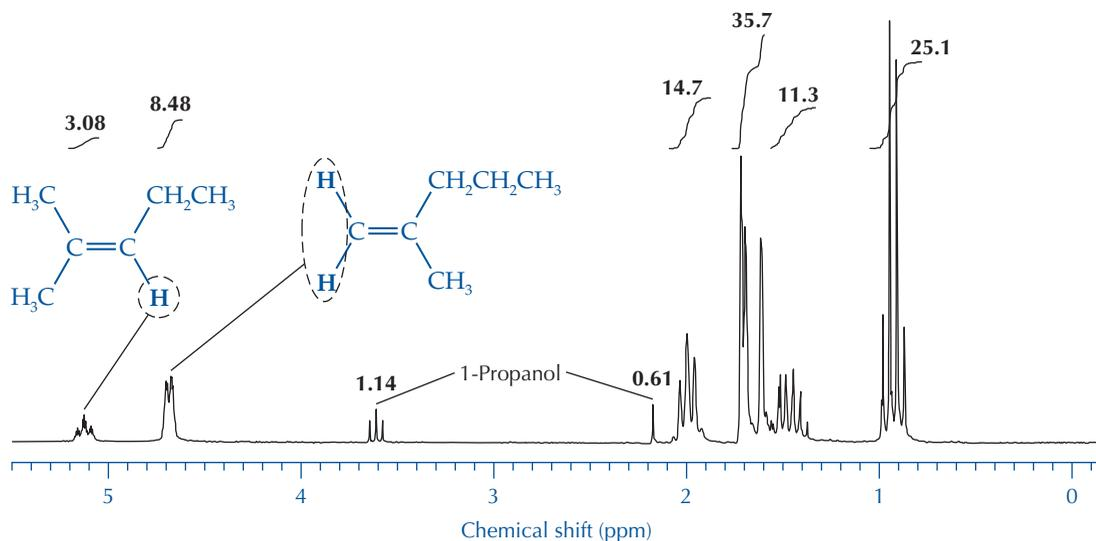
**FIGURE 21.29** 200-MHz  $^1\text{H}$  NMR spectrum of the reaction product from dehydrochlorination of 2-chloro-2-methylpentane, a mixture of 2-methyl-1-pentene and 2-methyl-2-pentene.
