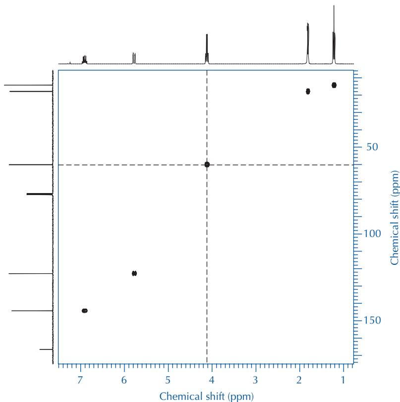
**FIGURE 22.14** 2D (C,H) COSY spectrum of ethyl *trans*-2-butenoate in  $\text{CDCl}_3$ . The 1D 360-MHz  $^1\text{H}$  NMR spectrum is shown at the top edge and the 90-MHz  $^{13}\text{C}$  NMR spectrum is shown at the left edge.
