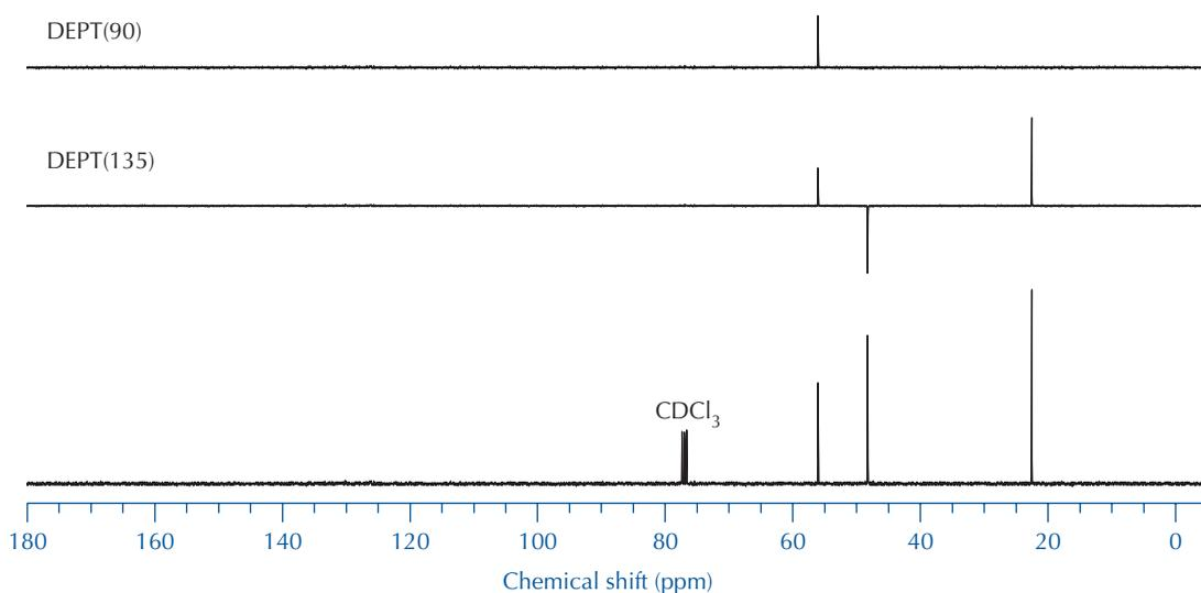
**FIGURE 25.6** 90-MHz  $^{13}\text{C}$  NMR, DEPT(90), and DEPT(135) spectra of unknown compound for problem 5.
