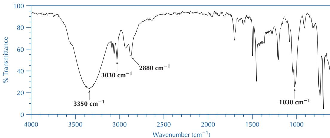
FIGURE 25.1 Infrared spectrum (thin film) of unknown compound for problem 2.
