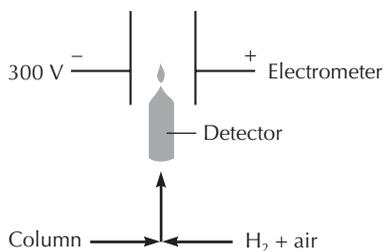
FIGURE 19.6 Flame ionization detector.
