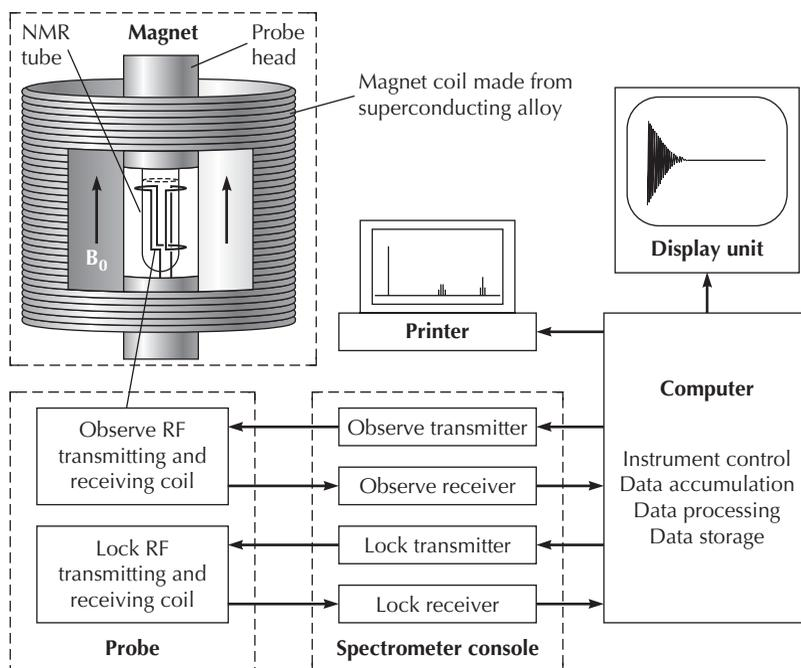
**FIGURE 21.5** Block diagram of a basic FT NMR spectrometer.
