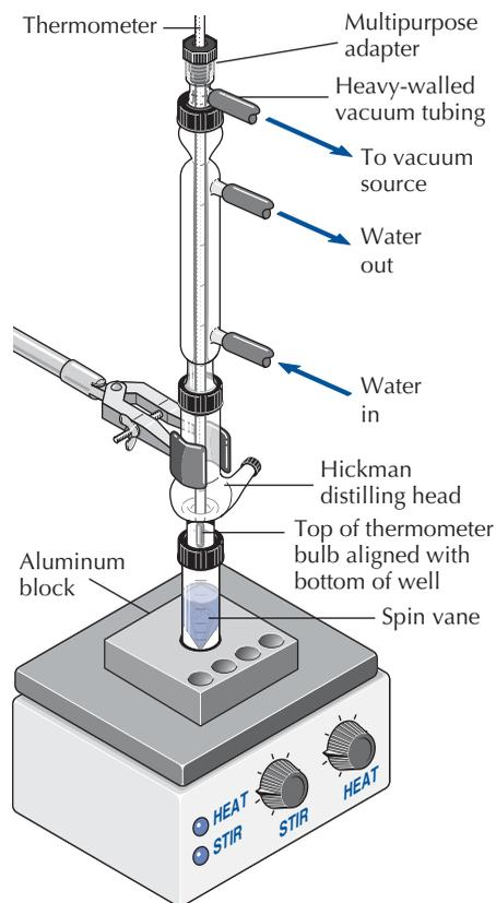
**FIGURE 13.29** Standard taper microscale apparatus for distillation with a Hickman distilling head.
