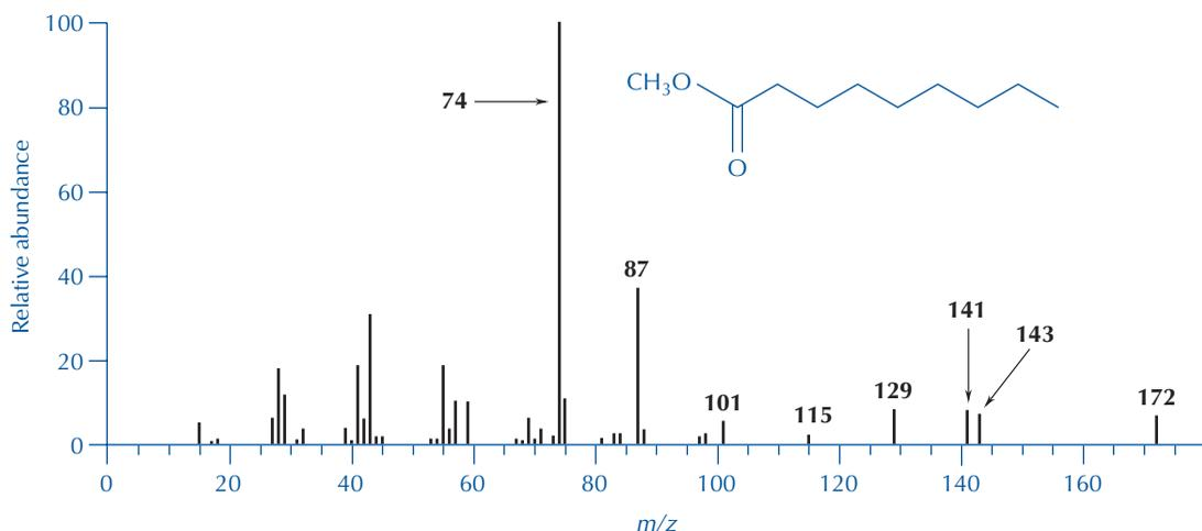
FIGURE 23.14 Mass spectrum of methyl nonanoate.
