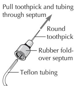
FIGURE 7.7 Threading Teflon tubing through a rubber septum.
