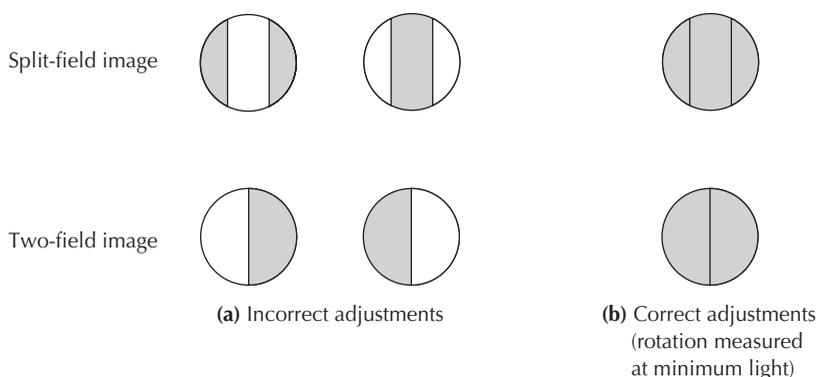
**FIGURE 16.5** Representative images in the light field of a manual polarimeter.
