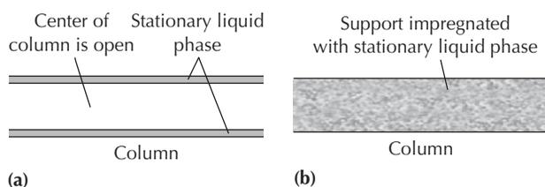
**FIGURE 19.1** Microview of (a) a wall-coated open tubular capillary column and (b) a packed column.
