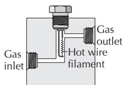
FIGURE 19.7 Thermal conductivity detector.
