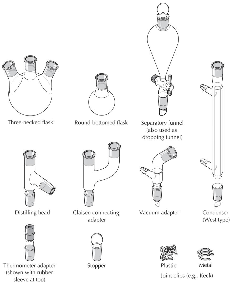
**FIGURE 4.4** Standard taper glassware for miniscale experiments.
