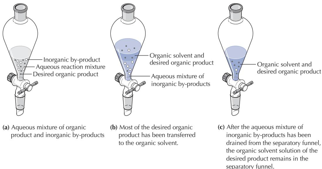
FIGURE 11.2 Using extraction to separate an organic compound from an aqueous mixture.
