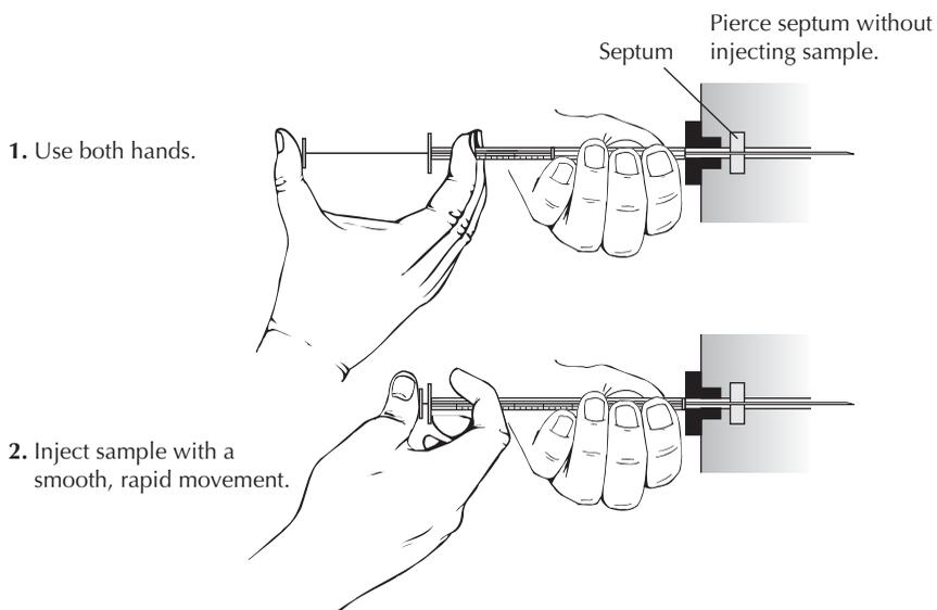
**FIGURE 19.10** Injecting the sample into the column.
