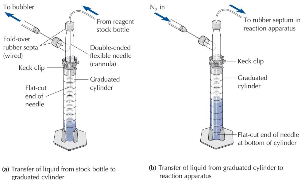
**FIGURE 16.12** Transfer of a liquid reagent (a) to a graduated cylinder and (b) from a graduated cylinder under inert atmosphere conditions.
