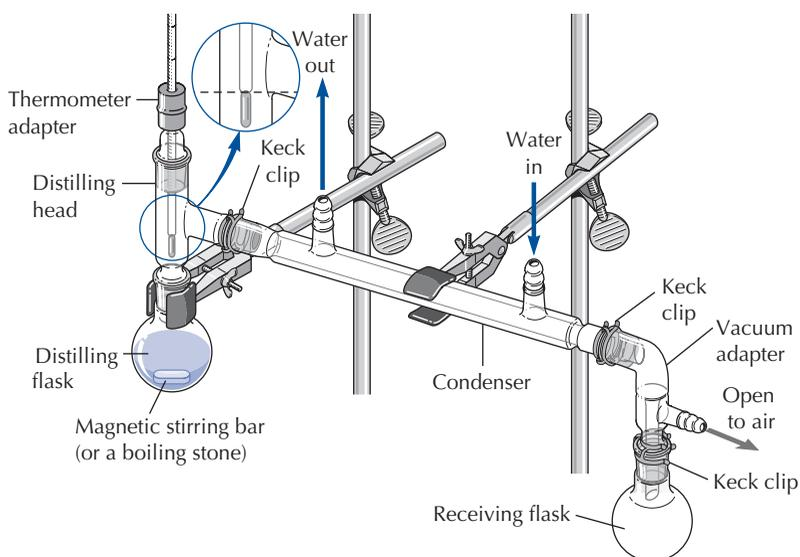
**FIGURE 13.7** Simple miniscale distillation apparatus. The enlargement shows the correct placement of a thermometer bulb for accurate measurement of the boiling point. If you are using a digital thermometer, consult your instructor about the correct placement of the temperature probe in the distilling head.
