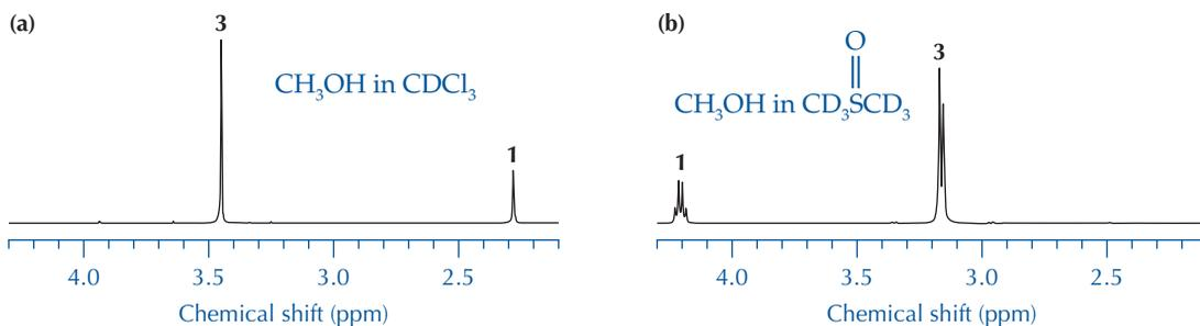
**FIGURE 21.32** 360-MHz  $^1\text{H}$  NMR spectra of methanol in (a) deuteriochloroform and (b) dimethyl sulfoxide- $d_6$ .
