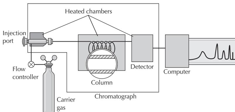
**FIGURE 19.3** Schematic diagram of a gas-liquid chromatograph.
