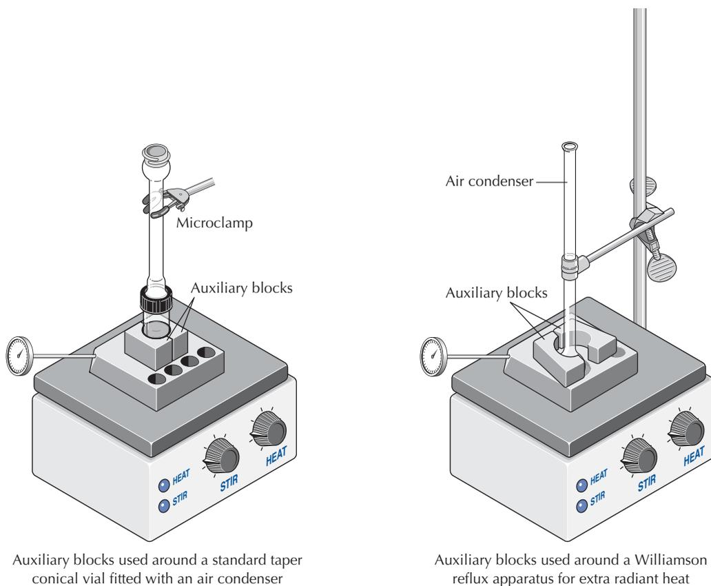
**FIGURE 6.3** Using auxiliary aluminum blocks to provide extra radiant heat with microscale glassware.
