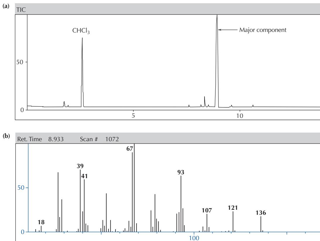
**FIGURE 23.5** (a) Total ion current gas chromatogram of orange oil. (b) Mass spectrum of the major component.
