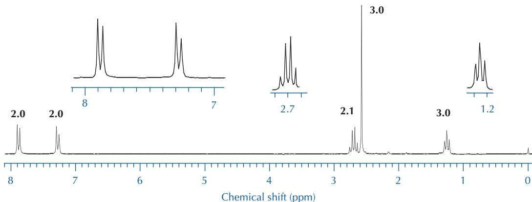
FIGURE 21.34 200-MHz  $^1\text{H}$  NMR spectrum of  $\text{C}_{10}\text{H}_{12}\text{O}$ .
