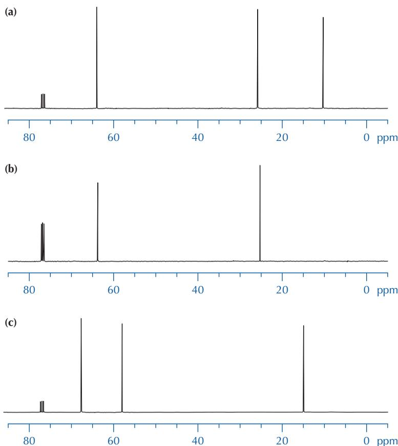
FIGURE 22.15 90-MHz  $^{13}\text{C}$  NMR spectra of compounds with molecular formula  $\text{C}_3\text{H}_8\text{O}$ .
