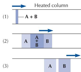
**FIGURE 19.2** Stages in the separation of a two-component (A, B) mixture as it moves through a packed column.
