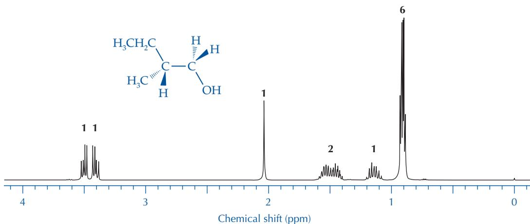
FIGURE 21.36  $^1\text{H}$  NMR spectrum of 2-methyl-1-butanol at 360 MHz.
