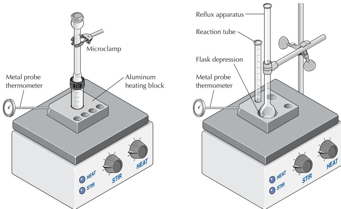
(a) Typical standard taper reaction apparatus with a conical vial and an air condenser
