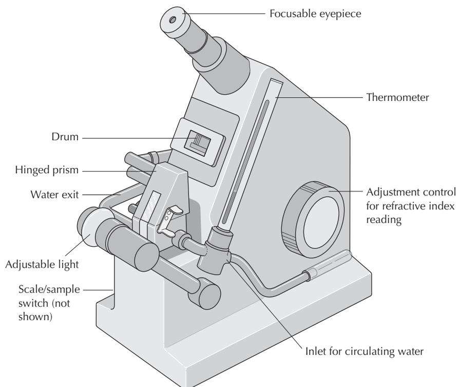
FIGURE 16.2 Abbé-3L refractometer.
