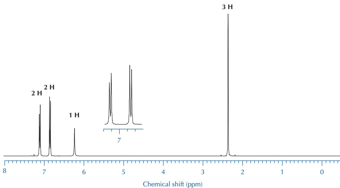
FIGURE 25.4 360-MHz  $^1\text{H}$  NMR spectrum of unknown compound for problem 4.
