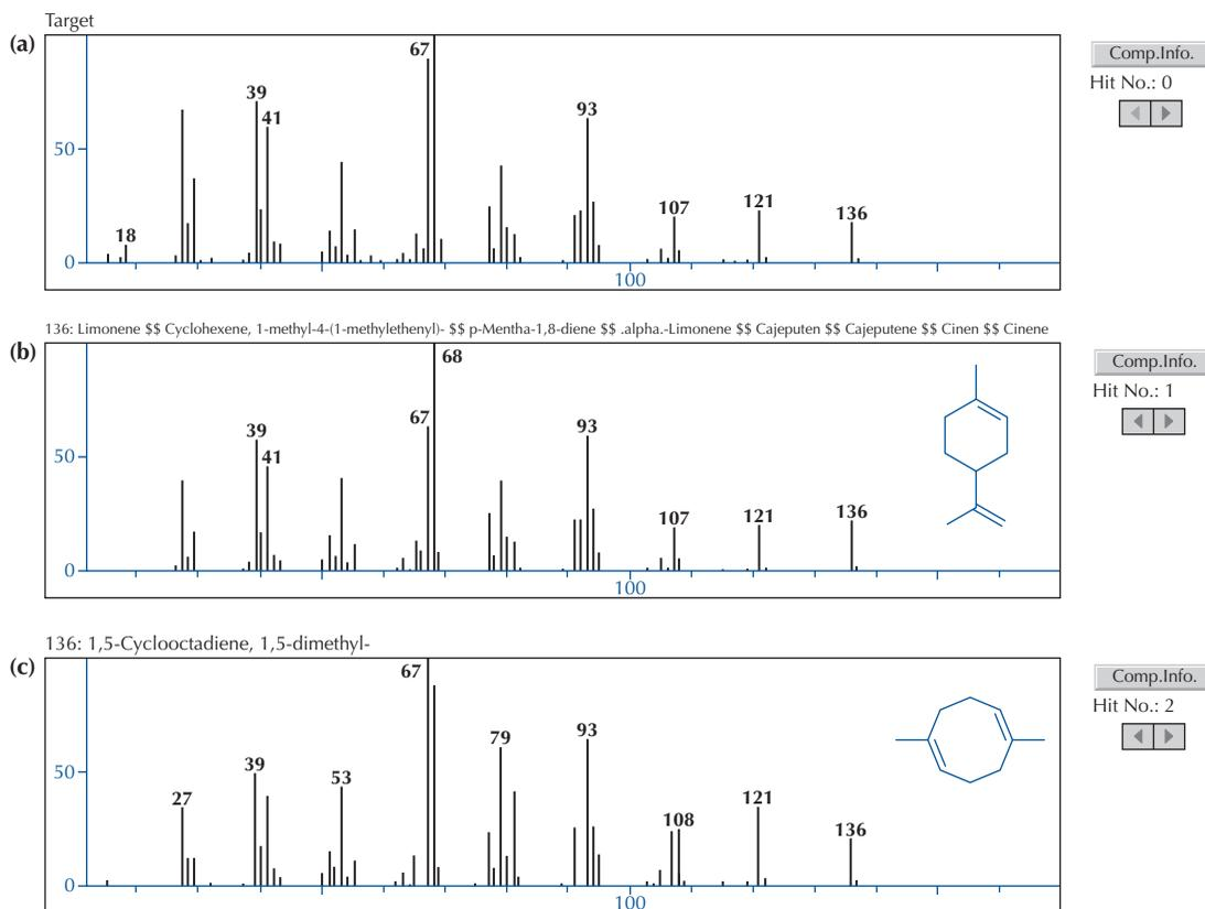
**FIGURE 23.10** Computer comparison of two hit-list compounds for orange oil. (a) MS of the compound from GC-MS run. (b) MS of hit 1. (c) MS of hit 2.
