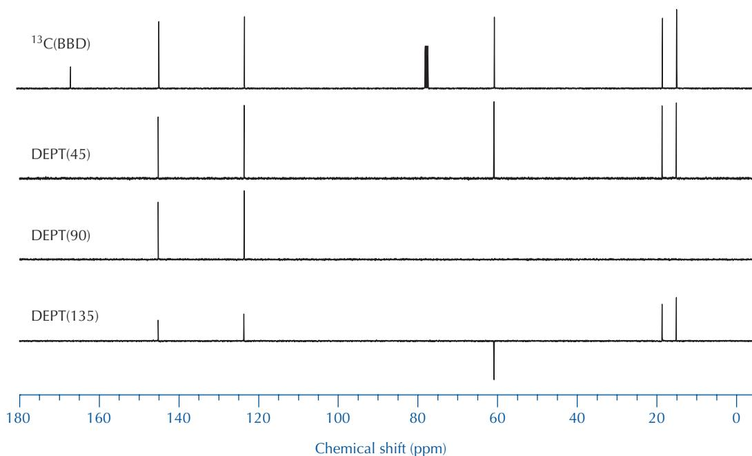
**FIGURE 22.11** DEPT spectra of ethyl *trans*-2-butenoate in  $\text{CDCl}_3$ . The broadband-decoupled 90-MHz  $^{13}\text{C}$  NMR spectrum is shown at the top.
