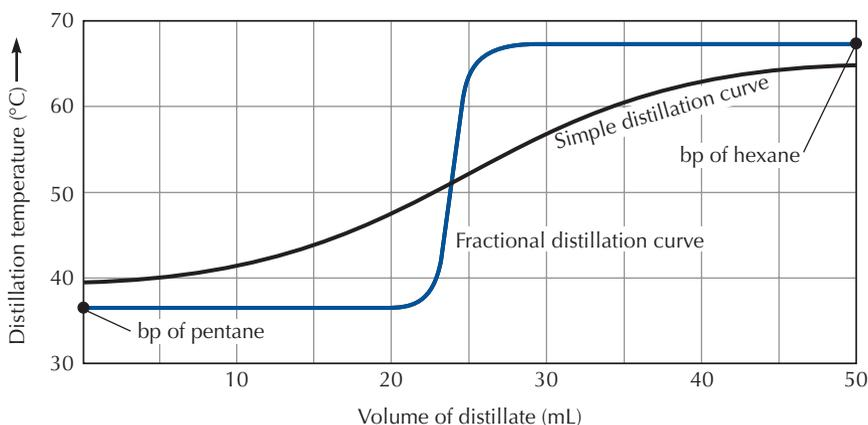
**FIGURE 13.16** Distillation curve for the fractional distillation of a solution of pentane and hexane. The dashed line represents the distillation curve for a simple distillation of the same solution.
