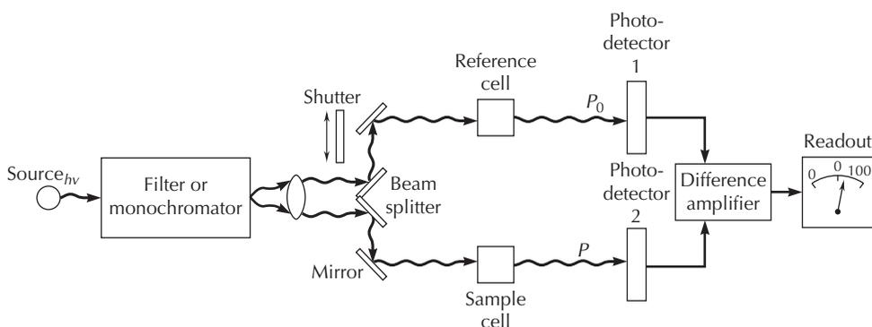
FIGURE 24.5 Schematic diagram of a double-beam spectrometer.
