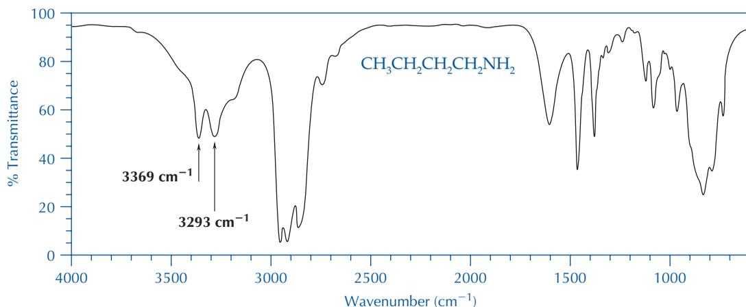
FIGURE 20.16 IR spectrum of 1-aminobutane (thin film).
