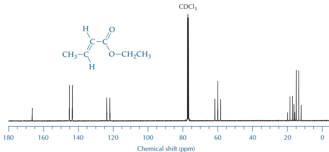
FIGURE 22.1 90-MHz  $^{13}\text{C}$  NMR spectrum of ethyl *trans*-2-butenoate in  $\text{CDCl}_3$ .
