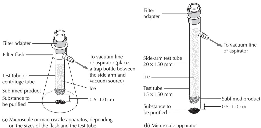
**FIGURE 16.1** Two simple apparatuses for sublimation.
