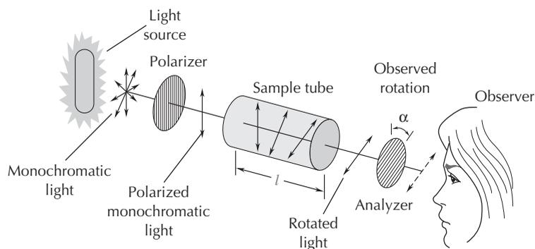
FIGURE 16.4 Schematic diagram of a polarimeter.
