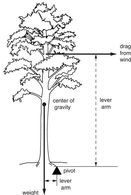
**FIGURE 1.4** The problem of a tree in a wind—the sideways force from drag acts far above the tree's base, so its drag causes a large turning force. That must be resisted by the tree's weight, with the small lever arm given by the radius of its base. (Attachment to the ground also helps a little.) The advantage of minimizing drag should be obvious.
