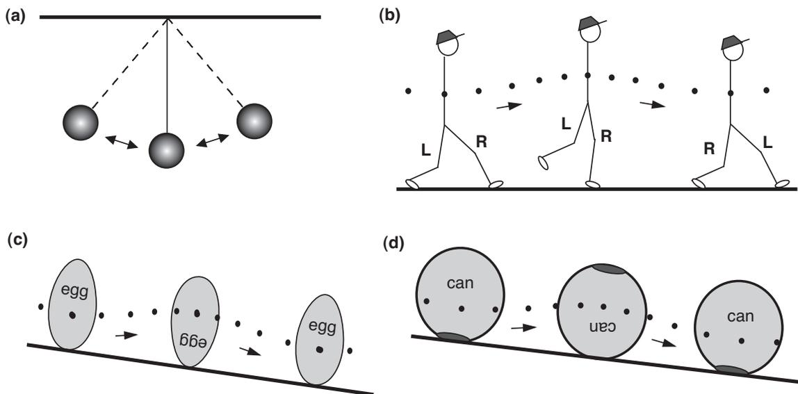
**FIGURE 1.1** (a) A conventional pendulum, (b) the inverted pendulum model for walking, (c) an egg rolling down an incline, and (d) a cylindrical can with an off-center weight rolling similarly. In (b), (c), and (d), the centers of gravity are shown as dark spots—their spacings (assume equal time between adjacent spots) give their velocities.
